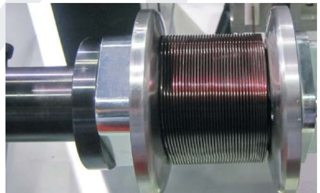
Typical edge wire wound coil with copper wire 5x20 mm
