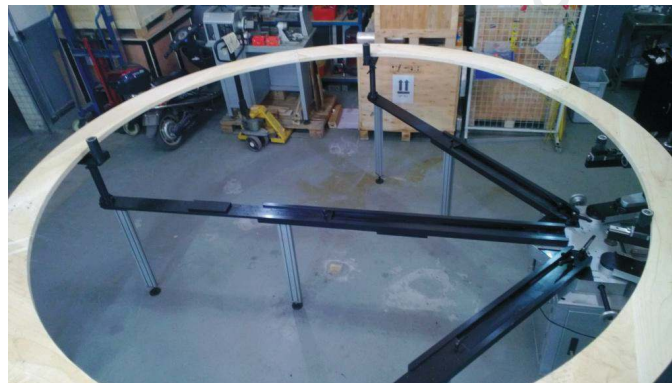
The Taping Machine with 4 metre large ring
