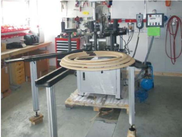
The VC-FLOOR Largest Horizontal Toroidal Taping Machine in the world
